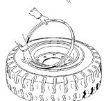
**4.** Put the lock ring in the correct position on the rim. Add air pressure to the tire as described in Add Air to Pneumatic Tires With Tube.
