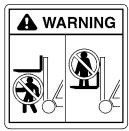
If a lift truck is used to elevate a worker, a safety platform must be attached to the forks and carriage. The platform must be specially built to meet or exceed the requirements of ANSI/ITSDF B56.1. It must have a solid floor with a surface to prevent the feet of the worker from slipping, hand rail, toe board, and a screen or
