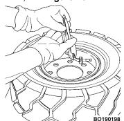
2. Put wheel and tire assembly on the press. Position the feet of the press on the loose flange. Push press down on loose flange to expose the locking ring.
