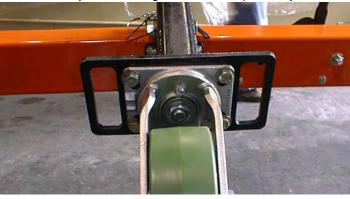
Lube Point(s) - 1 Grease Fittings Capacity - As Required Lube - MPG Interval - As Required
