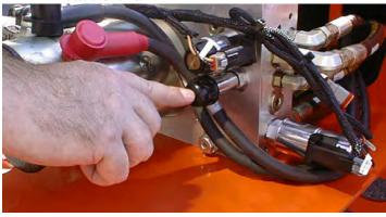
**2.** Locate the hand pump located on the front face of the valve block, the handle is loose mounted to the valve mounting plate.
