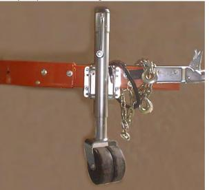
**5.** Remove the pin securing the jockey wheel in the drive position and swing the wheel up into the stowed position. Secure the wheel in place with the retaining pin.
