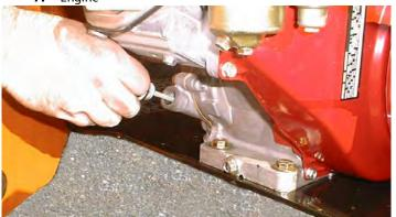
Capacity - See Engine Manual. Lube - EO, 10W30 API SJ Interval - Check level daily; change per manufacturer's engine manual. Comments - Adjust final oil level by mark on dipstick 8. Fuel Tank
