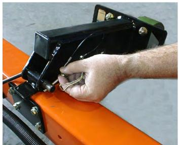
Pull out on the drive & set control valve knob. Ensure friction wheels are disengaged from tires.
