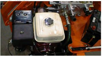
Capacity - 1.6 Gal. (6.0 L) Fuel - Gasoline Interval - Check periodically during each shift
