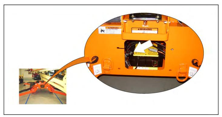
Figure 5-5. Generator Plug Location
