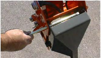
**6.** Remove the platform console from the platform and connect the console harness to the receptacle at the hook storage area on the turntable.
