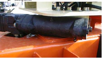
Lube Point(s) - 2 Grease Fittings Capacity - As Required Lube - MPG Interval - As Required
