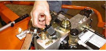
**NOTE:** The cap securing the filter must be torqued 154 to 170 ft.lbs. (209 to 230.5 Nm).
