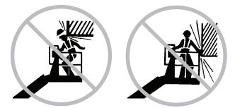
Be aware of crushing hazard when grasping the platform guard rail.
