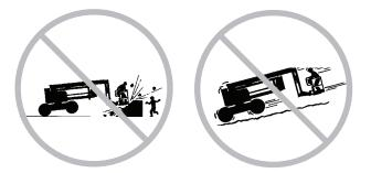
Limit travel speed according to condition of ground surface, congestion, slope, location of personnel, and any other factors which may cause collision.
