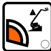
**S-80 HF, S-85 HF:** The range of motion light is on when the platform load is less than 600 lbs/272 kg and on a slope
