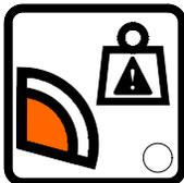
**S-80 HF, S-85 HF:** The range of motion light is on when the platform load exceeds 600 lbs/272 kg.
