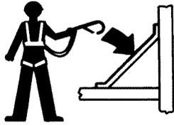
Occupants must wear a safety belt or harness in accordance with governmental regulations. Attach the lanyard to the anchor provided in the platform.
