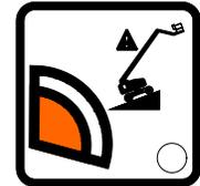
10 Machine on incline indicator light
