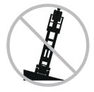
If the tilt alarm sounds: Lower the mast, then lower the jib boom. Move the machine to a firm, level surface. Use extreme caution to lower the mast.
