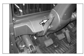
1. Engage the parking brake, if not already engaged. Place the transmission directional control lever in the NEUTRAL position.
