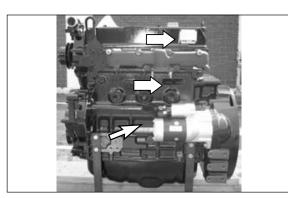
3.3 liter Diesel Engine (4TNE98) Serial Number
