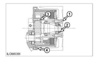
Torque for wheel bolts (1) is 270  $\pm$  25 N•m (200  $\pm$  20 lb•ft).
