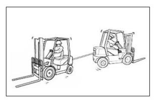
The counterweight draw bar should not be used for towing the forklift or for towing another forklift. Towing is only advised in emergencies, by trained operators and at low speed, no faster than 2 km/h, to a convenient location for repair.
