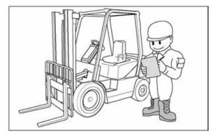
Inspect and check the condition of your forklift truck using the operator's check list before starting work. Immediately report to your supervisor any obvious defects or required repairs.
