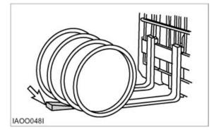
1. Block drums or round objects. Tilt the mast FORWARD and slide the fork tips along the floor to get under the load.
