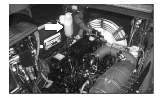
**12.** Observe the engine coolant level in the coolant recovery bottle. With the engine cold, maintain the level to the COLD mark. If the recovery bottle is empty, also fill the radiator at the top tank.
