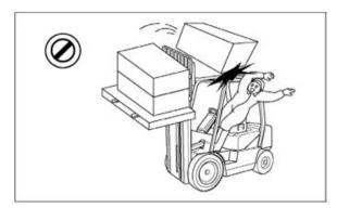
Do not move loose loads that are higher than the load backrest.
