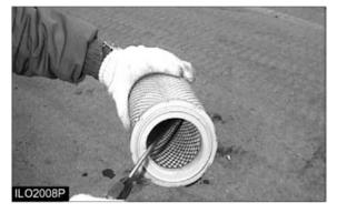
Direct air on the inside and outside of the element along the length of the pleats. Check the element for any tears, rips or damage
