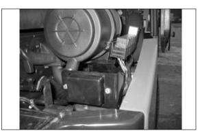
Remove the front cover from the fuse box located under the cowl.
