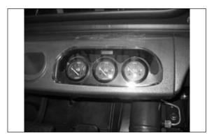
**13.** Observe the fuel level gauge after starting the truck. Add fuel if necessary.
