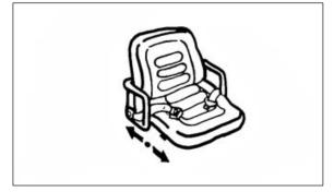
Adjust the seat before operating the lift truck. After adjusting, set the seat to make sure it is properly locked. Do not adjust the seat while the truck is in motion.
