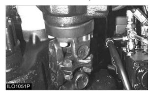
Check for worn or damaged bearings. Have worn or damaged bearings replaced. Check for loose retaining bolts and nuts. Tighten the bolts and nuts, if necessary.
