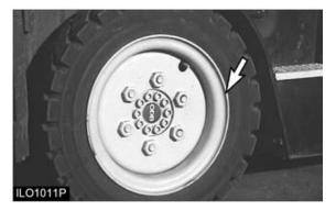
Do not re-inflate a tire that has been run while flat or underinflated, without first checking to make sure the locking ring on the rim is not damaged and is in the correct position.
