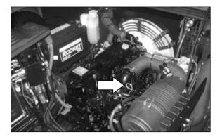
**11.** Measure the engine crankcase oil level with the dip stick. Maintain the oil level between the MAX. and MIN., (or FULL and ADD) notches on the dip stick.
