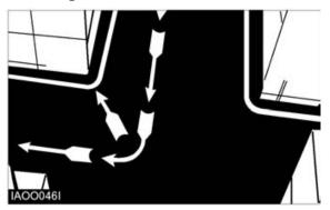
1. When turning sharp corners, keep close to the inside corner. Begin the turn when the inside drive wheel meets the corner.
