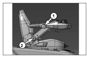
By using 2 knobs, adjust the position of the armrest to give the operator the best comfortable position of arm.
