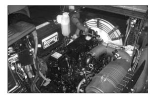
**10.** Inspect the engine compartment for oil, coolant and fuel leaks.
