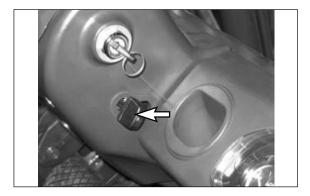
To adjust the steering column, push down the knob(1), and move the steering column to the desired position, then release the knob(1).
