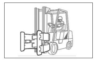
There are many special attachments available to replace the forks on a lift truck.
