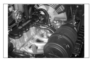
Service the air cleaner when the red target in the service indicator stays locked in the visible position with the engine stopped.
