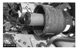
2. Remove the secondary element. Inspect the gasket between the air cleaner housing and the engine inlet. Replace the gasket if it is damaged.
