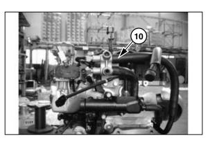
**10.** Remove the indicated coolant hose above picture and then, add the coolant to hose as much as needed.
