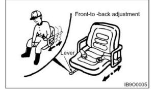
Move the lever, slide the seat to the desired position, and release the lever.
