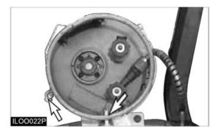
**11.** Position the replacement tank so that the locating pin (dowel) is in place.
