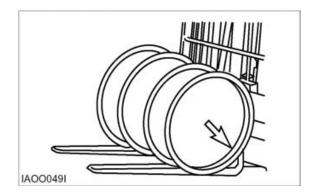
**2.** Before lifting, tilt the mast BACK slightly until the load is cradled on the forks.
