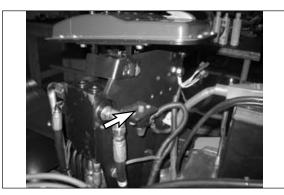
**Circuit Breaker** -Protects the main electrical circuits. To reset the circuit breaker, push the button in. Located in the engine compartment.
