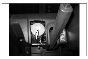
The brake reservoir is located on the left side of the steering column.
