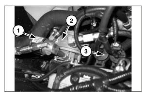
(1) LP fuel lock-off(2) Regulator/Converter(3) Fuel Trim valve (FTV)
