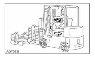
Use special care when operating on grades. Do not angle across or turn on grades. Do not use lift truck on slippery grades. Travel with forks downgrade when unloaded. Travel with load upgrade.
