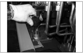
**3.** Remove the dip stick/filter cap. Maintain the oil level to the FULL mark on the dip stick/filter cap.
