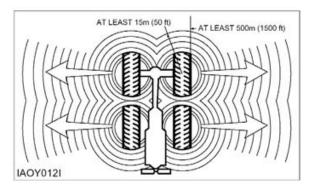
Do not approach a warm tire closer than the outside of the area represented by the shaded area in the above drawing.
