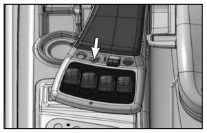
In case of auto tilt leveling, push this button. Pushing button makes auto tilt leveling function on and off alternately. When the function is on, the mast stops at a vertical position while tilting forward and backward.
