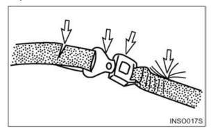
1. If the seat belt is torn, if pulling motion is interrupted during extension of the belt, or if the belt cannot be inserted into the buckle properly, replace the seat belt assembly.
