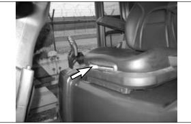
1. Check the operation of the seat adjuster rod. Make sure that the seat slides freely on its track.
