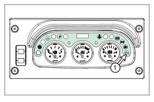
(1) Malfunction Indicator Lamp(MIL) for Engine control system.
