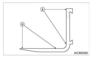
Check the straightness of the upper face of blade (D) and the front face of shank (E) with a straight edge.
