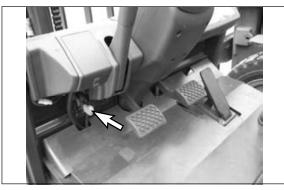
1. The engine compartment is accessible by pulling the latch (GC Series), or pushing down the lever located at cowl (G.D Series) and raising the hood and seat assembly (Note: Unlock latch before pulling-if key equipped)
