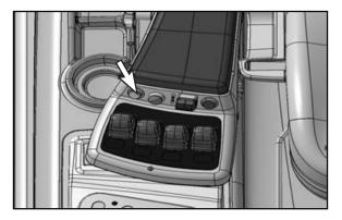
The state of the finger tip system can be checked by the external warning lamp blinking..
