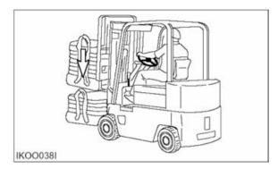
Tilt the elevated load forward only when directly over unloading area and with load as low as possible.
