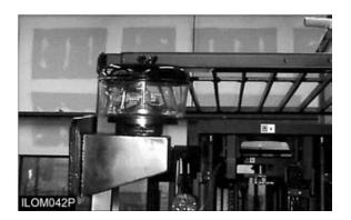
1. Check the precleaner bowl for dirt build-up. If the dirt is up to the line, remove the precleaner bowl and empty it. Periodically wash the cover and bowl in water.
