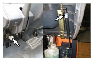
1. Raise the hood and seat assembly. Make sure the support cylinder securely holds the hood open.
