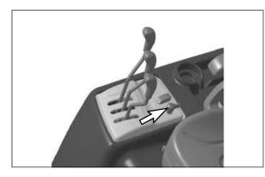
**2.** Lift trucks equipped with electrical disconnect switches; the engine will not start unless the disconnect switch is in the ON (closed) position.
