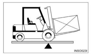
Counterbalanced lift truck design is based on the balance of two weights on opposite sides of a fulcrum (the front axle). The load on the forks must be balanced by the weight of the lift truck. The location of the center of gravity of both the truck and the load is also a factor. This basic principle is used for picking up a load. The ability of the lift truck to handle a load is discussed in terms of center of gravity and both forward and sideways stability.
