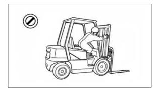
Do not operate a lift truck unless you are in the operator's seat. Keep hands and feet inside the operator's compartment. Do not put any part of the body outside of the operator's compartment. Never put any part of body into the mast structure or between the mast and the truck
