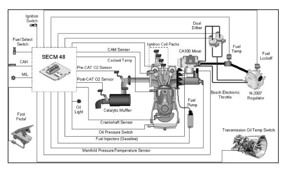
EMS schematic of G420FE / G424FE / G424IE Dual fuel engine
