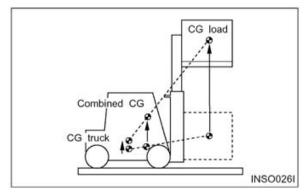
These same factors are also important for unloaded lift trucks. They tip over sideways easier than a loaded lift truck carrying its load in the lowered position.
