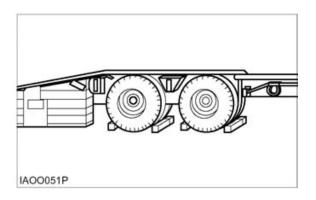
Always block the trailer or the rail car wheels before loading the lift truck.
