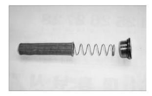
**2.** Wash the strainer assembly in clean, nonflammable solvent and dry it. Install the strainer assembly.
