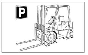
Park your lift truck in authorized areas only. Fully lower the forks to the floor, put direction lever in NEUTRAL position, engage the parking brake, and turn the key to the OFF position. Remove the key and put blocks behind the wheels to prevent the truck from rolling. Shut off your forklift truck when leaving it unattended.
