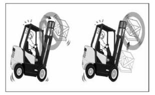
Do not elevate the load with the mast tilted forward. Do not tilt the elevated loads forwards. This will cause the lift truck to tip over forward.
