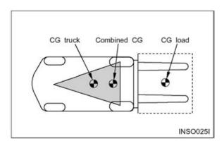
The stability of the lift truck is determined by the location of its CG; or, if the truck is loaded, the combined CG of the truck and load. The lift truck has moving parts and, therefore, has a CG that moves. The CG moves forward or backward as the mast is tilted forward or backward. The CG moves up or down as the mast moves up or down. The CG and, therefore, the stability of the loaded lift truck, are affected by a number of factors such as:
