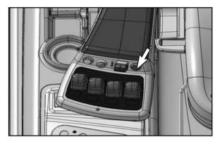
In case of emergency, push this button. Pushing button makes the finger tip system on and off alternately. So if the finger tip control dose not work, then press this button once.
