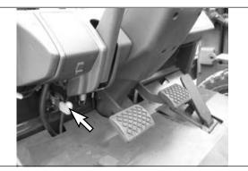
Push the lever down to raise the hood and seat assembly. Make certain the support cylinder will hold the hood open.
