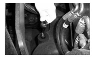
7. Install the dip stick/filter cap.
