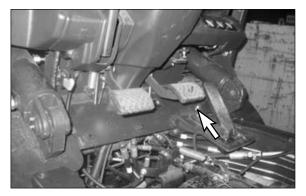
1. Lubricate three fittings for the inching and brake pedal control shaft.
