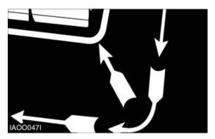
2. In narrow aisles, keep away from the stockpile when turning into the aisle. Allow for counter weight swing.
