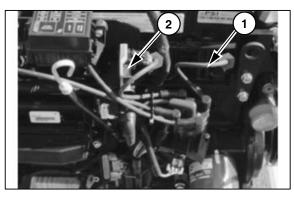
(1) Spark Plug Cables(2) Ignition Coil
