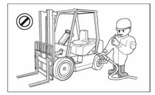
Forklift trucks may only be refueled at specially reserved locations. Switch off the engine when refueling.
