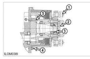
Torque for single or dual wheel mounting nuts (1) is  $644 \pm 34$  N•m (470  $\pm 25$  lb•ft).
