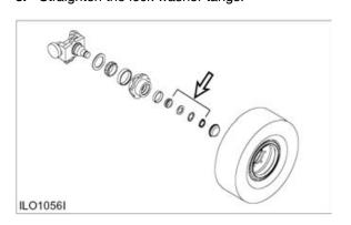
Remove the locknut, lock washer and flat washer. Remove the outer wheel bearing.
