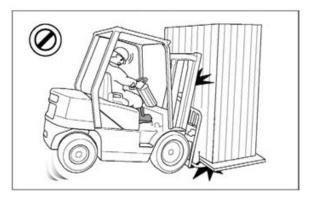
Do not overload. Always handle loads within the rated capacity shown on the capacity plate. Do not add extra counterweight to the truck. An overload can cause the truck to roll over and cause injury to personnel and damage to the lift truck.
