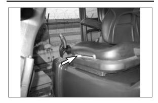
**14.** To position the seat, PUSH the lever away from the seat track and move the seat forward or backward to a comfortable position.
