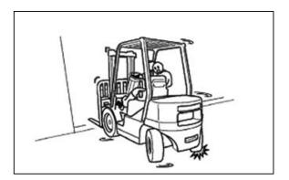
An unloaded forklift may be easier to tip over than a loaded truck.
