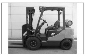
1. Park the lift truck only at a designated safe location. Place the transmission in NEUTRAL. Lower the forks to the ground. Engage the parking brake. Stop the engine.
