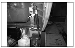
2. The hood and seat assembly is held up by a support cylinder. Make certain the air cylinder is operating properly and securely hold the hood up before doing anything in the engine compartment.
