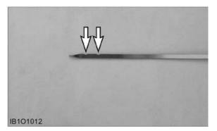
1. Maintain oil level between the MAX. and MIN. marks on the dipstick.
