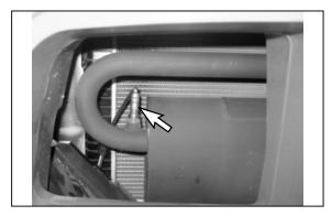
When indicated by MIL, replace oxygen seasor on the exhaust manifold and oxygen sensor on muffler assembly.
