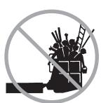
Do not place ladders or scaffolds in the platform or against any part of this machine. Do not transport tools and materials unless they are evenly distributed and can be safely handled by person(s) in the platform.
