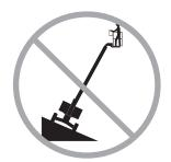
Do not raise or extend the boom unless the machine is on a firm, level surface.
