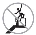
Do not sit, stand or climb on the platform guard rails. Maintain a firm footing on the platform floor at all times.
