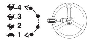
Come to a complete stop before shifting the transmission from forward to reverse. The transmission control lever must be in 1st or 2nd gear only.
