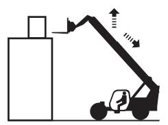
When the forks are clear of the load and the structure, the boom can be lowered and retracted.
