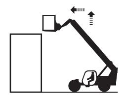
6 Gradually move the controller to lower and extend the boom into final position. Lower the load until the weight is completely off the forks. Do not apply a downward force with the forks.
