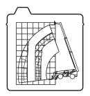
Occupants, equipment and materials shall not exceed the maximum platform capacity. Distribute loads evenly on the platform floor.
